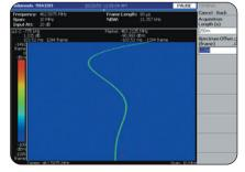
RSA Series Spectrogram uniquely shows time-varying signal behavior in frequency change/stability, spectrum occupancy, pulsed signal timing, power change and more! The sample above shows the frequency settling characteristic of a transmitting device.
