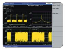
Time-correlated multi-domain view provides a new level of insight about design or operational problems and possible solutions. This example includes frequency, time, and modulation domain views of an AM-modulated pulsed signal with pulseto-pulse phase variation measured in the modulation domain.
